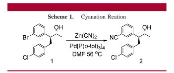
$Zn(CN)_2$  at 56 °C for 16 h. A sample of each was then filtered to remove undissolved  $Zn(CN)_2$ , and the solution was assayed for soluble cyanide using ion chromatography (IC), Table 1.<sup>6</sup>
